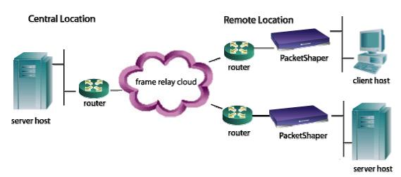
PacketShaper sits behind WAN-link routers and alleviates the performance degradation that results from bandwidth bottlenecks. Branch offices and remote sites benefit most from PacketShaper; it makes efficient use of a limited-capacity link, increases throughput, and protects critical applications.
